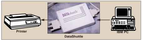
DataShuttle attaches to your PC through a high speed parallel pass-thru interface, so you don't have to disconnect your printer.
